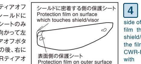
3 After adjusting the tension, detach the CWR-F2R tear-off film from the shield/visor and once again remove any dust or oil adhered to the surface of the shield/visor.
