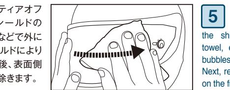
5 Securely attach the CWR-F2R tear-off film to the shield/visor while using a towel, etc. to push out any air bubbles between the two surfaces. Next, remove the protective sheet on the front surface.
