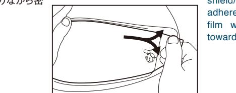
4 Peel off only the protective sheet on the side of the CWR-F2R tear-off film that will adhere to the shield/visor and then attach the film starting from the left CWR-F2R tear-off button with reference to the shield/visor. After this, adhere the CWR-F2R tear-off film while lightly pulling it toward the right.
