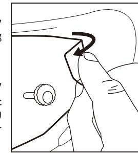
7 To make the CWR-F2R tear-off film easier to remove, gently fold the slightly longer part of its front right edge toward you.
